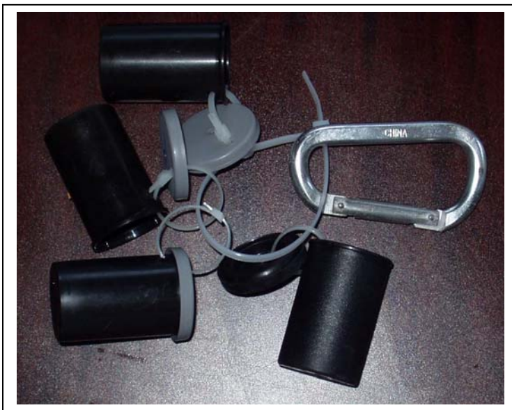
Figure 1. Basic configuration design of 35 mm film canister loop for coral sampling
