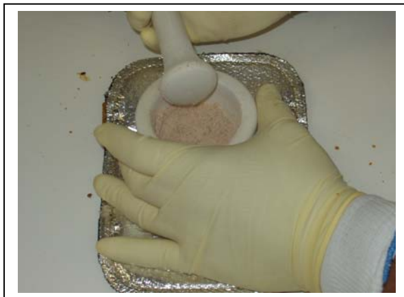
Figure 15. Grind samples into a fine powder, making sure that the sample never thaws. Be careful when pouring liquid nitrogen into the mortar with granulated sample, as the liquid will sometime splash the sample out of the mortar and onto the bench.
