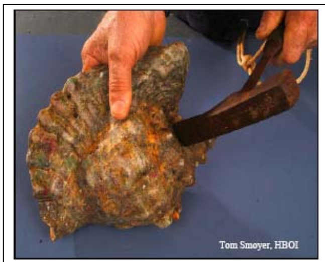
Figure 5. Puncture or “crack” the shell at the location indicated in the figure. Use an acetone-cleaned stainless steel hammer with a spar or a stainless steel chisel.
